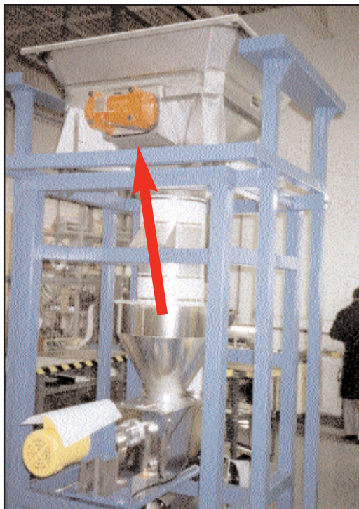
SCR-300 on Box Dumper to prevent hang-ups.
